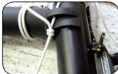
A square knot to help adjusting the preventer.
