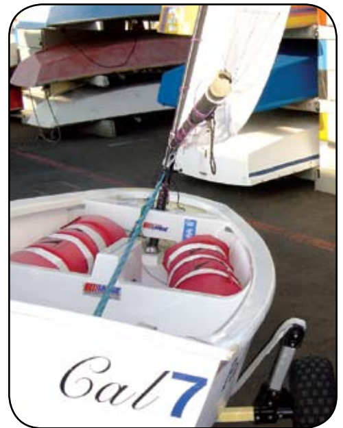
Boom should align with the corner of the boat
